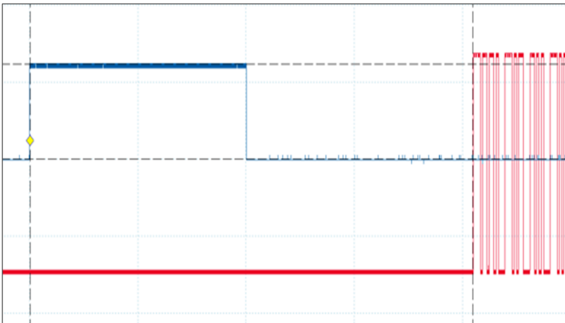
Figure 7-5: Configuration 2: Timing offset=20ms. 1PPS in blue and NMEA messages in red.
