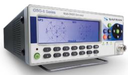
Simulation is simply the best way to test and verify proper operation of devices, systems and software reliant on global navigation satellite signals. Orolia GSG-5/6 series simulators are easy to use, feature-rich and affordable to offer the best value compared to alternative testing tools or the limitations of testing from "live sky" signals.
