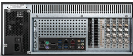
A CDM-5 is shown here synchronizing SDRs in a Skydel SDX GNSS Simulator System
