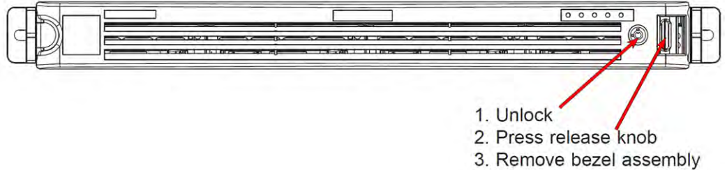
Figure 4-13: Removing the front bezel
