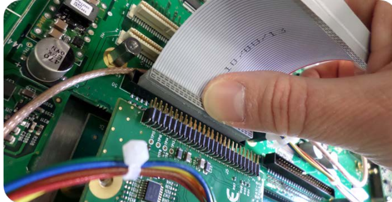
Figure 5-5: Ribbon cable installation
