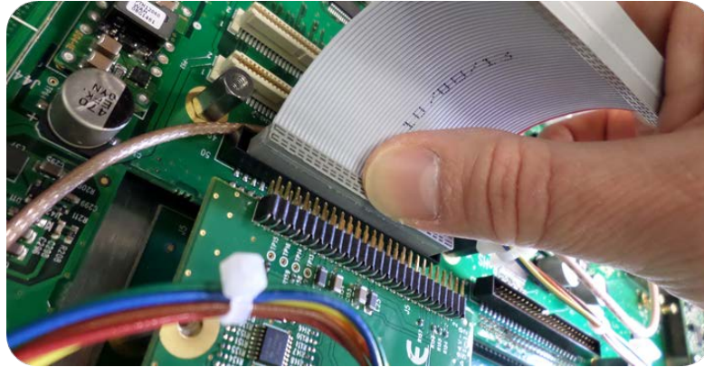
Figure 5-7: Ribbon cable installation
