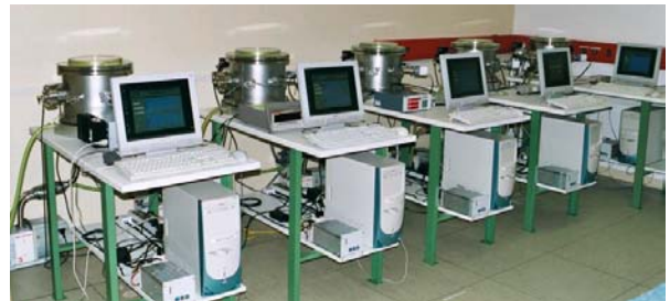
Figure 2. Five EQMs without external cover and vacuum chambers for life test with 'Picotime' measurement systems
